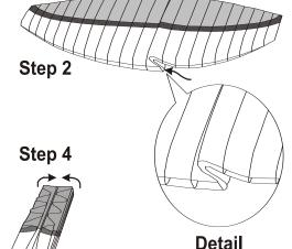
In order to prolong the life of the ASS battens we recommend the following procedure when folding the canopy in the chord-wise direction:
