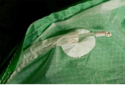
Push the batten back somewhat and release the end from the pocket, then remove it entirely. Transfer the total length precisely to the replacement material (supplied) and cut a new length. File the ends of the new batten and cover them with tape. Push the new batten into place and secure.
