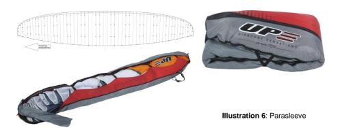
Now your wing is in a neat but long package. Fold the trailing edge around 30cm in, and fold the leading edge on top of the fold, click the final buckles and you're done. If you are storing your UP Kangri for extended periods we recommend packing using the ParaSleeve method. Also, on rugged/abrasive surfaces we suggest that you adapt the packing method to be able to leave the wing on the ParaSleeve all the way through, to avoid mechanical abrasion.
