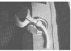
Should this be the case we recommend the use of a small piece of cotton thread between the locking pin and the closing loop on the reserve container (see illustration). This is a simple, cheap and efficient way to eliminate involuntary deployments, but always take care to test the system on the ground before flying with it.
