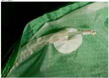
Use the damaged batten to measure a perfect new one from the extra batten material. The new ends should be sanded/filed round/ and covered with woven sticky tape before use. When inserting the new batten, make sure it is
