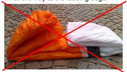
Do NOT fold the leading edge under, as shown here above.
