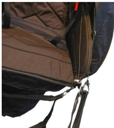
On the left hand side the line goes first through the metal pulley, then the grommet in the leg cover and then it is tied onto the plastic buckle.
