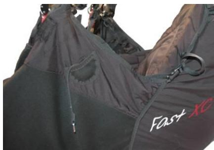
From there they are threaded through the ball-bearing pulley. From the pulley the lines go on the INSIDE of the main suspension system of the harness, down through the lateral pulleys at the end of the seat plate and to the speed bar.
