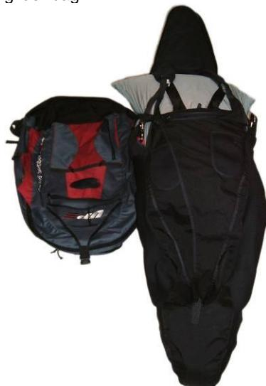
Open the glider rucksack and place the package on it, the back side downwards.
