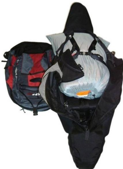
Close the leg cover around the glider so that it isn't unduly wrinkled in the glider bag.
