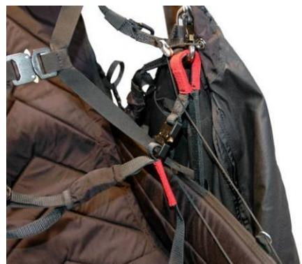
Adjust the line so that the nose of the leg cover does not touch the ground during the launching phase. At the same time, make sure the harness is closed cleanly when the flying position has been reached in flight.
