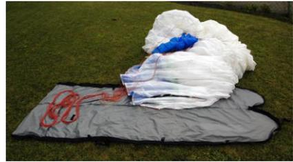
Sit on the opposite side of the bag and pull the cells onto the bag, one by one, from the nearest stabilo, across the middle and to the furthest stabile.
