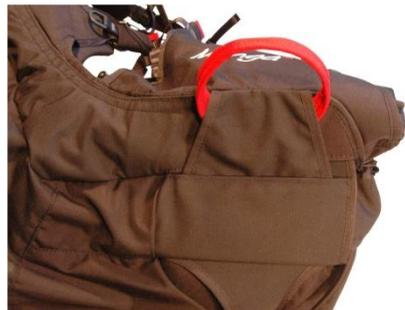
Then stick the top container flap through the deployment handle and secure it with the Velcro.
