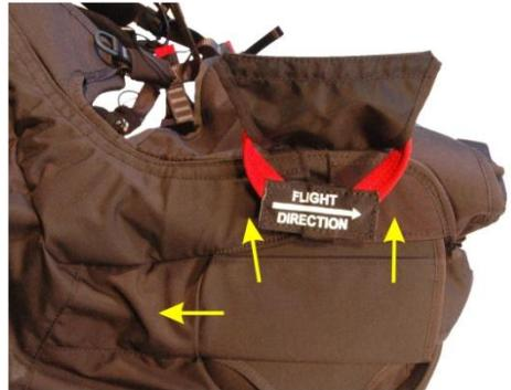
Pull the lower container flap upwards and slide it into the pocket beneath the deployment handle.
