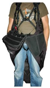
The speed bar lines go through the lateral neoprene slits of the leg cover.
